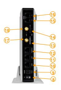
1. Power LED 2. LAN0 LED 3. LAN1 LED 4. GSM Port 0 LED 5. GSM Port 1 LED 6. Analog Port 2 LED 7. Analog Port 3 LED 8. Power On/Off Switch 9. Power Adaptor Input 10.10/100Mbps LAN0 Interface 11.10/100Mbps LAN1 Interface 12.Console Port 13.SIM Card Slot 0 14.SIM Card Slot 1 15.Analog Port 0 (FXS, FXO) 16.Analog Port 1 (FXS, FXO) 17.GSM Port 0 Antenna 18.GSM Port 1 Antenna
