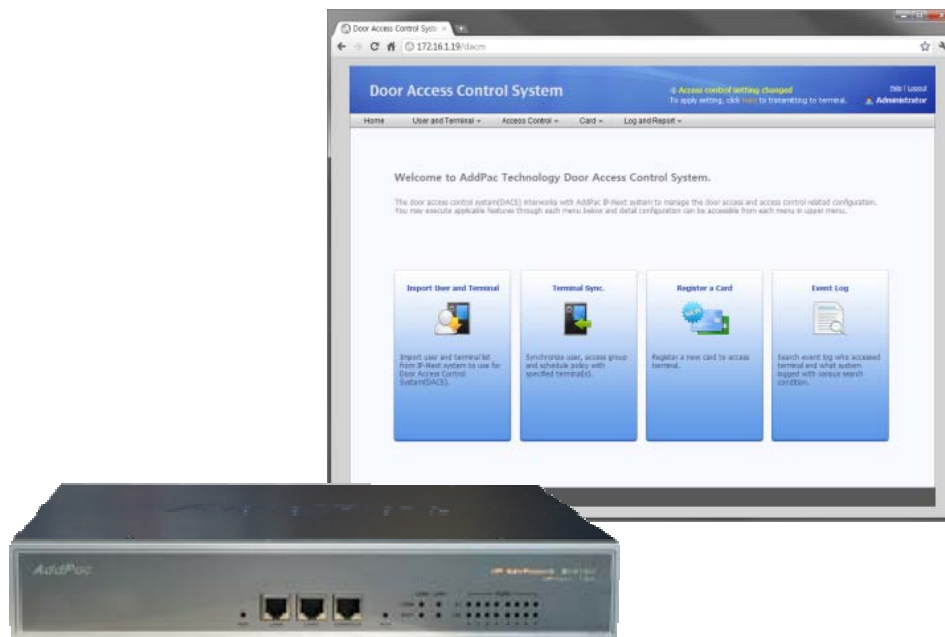
AP-ACS1000 Door Access Control Server (Call Manager + Door Access Controller)
