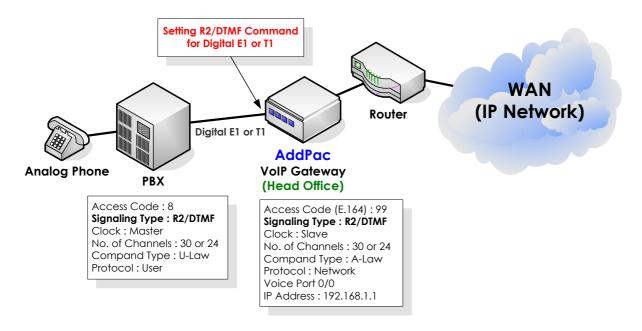
(Figure 2-3) R2/DTMF Network Diagram
