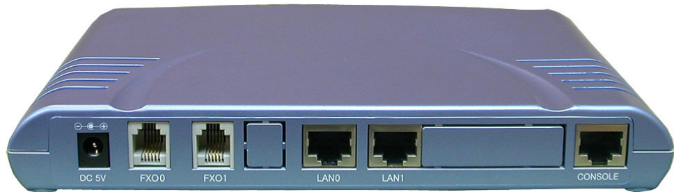
Figure 1-7: The rear panel of VoiceFinder AP200D model
