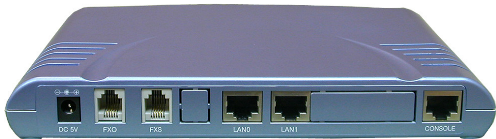
Figure 1-8: The rear panel of VoiceFinder AP200E model
