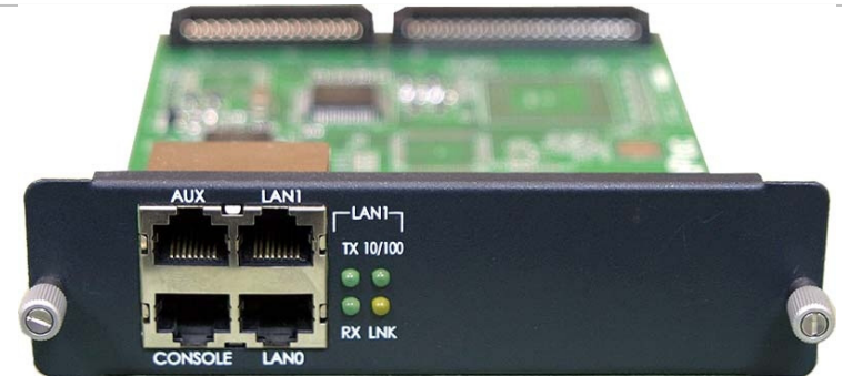
2-Port 10/100Mbps Fast Ethernet Interface 2-Port Asynchronous Serial Interface
