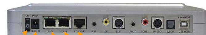
[Power SW] [Ext. Power Input] [LAN0 10/100Mbps Ethernet] [RS-232C Console] [LAN1 10/100Mbps Ethernet]
