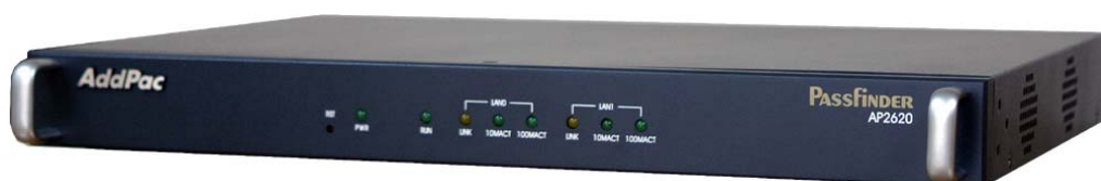
[ Figure 1-2 The Exterior of VoiceFinder AP2620 VoIP Gateway ]
